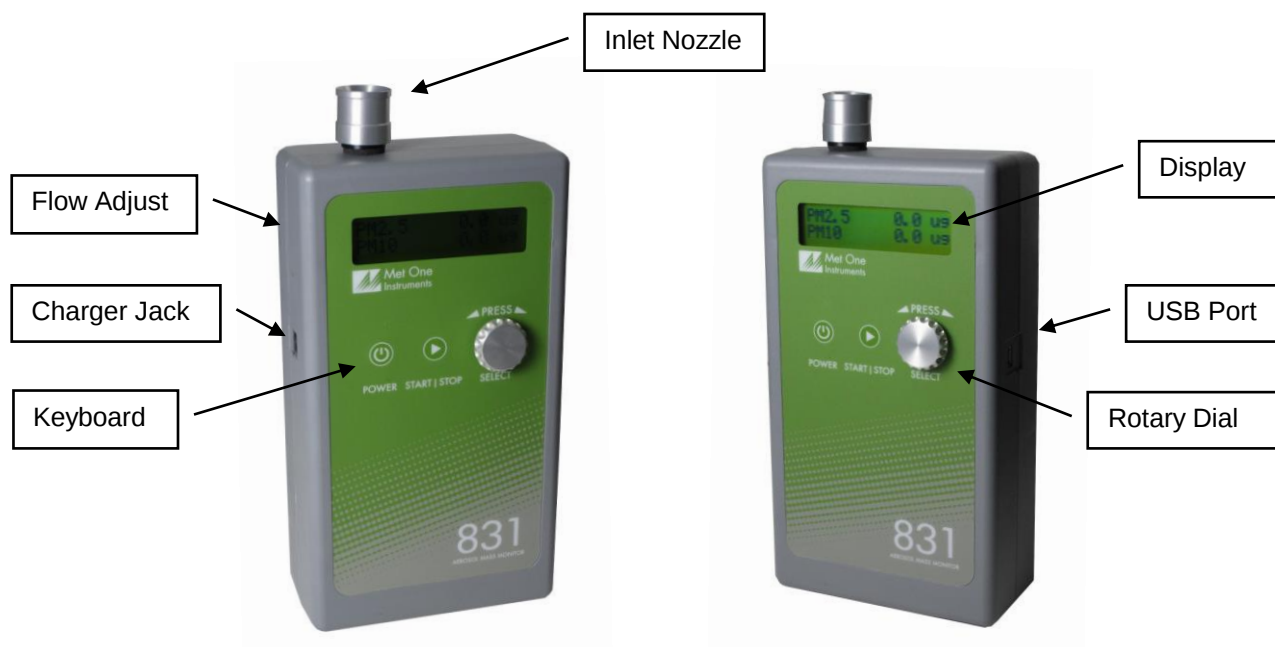
Figure 3 – AEROCET 831 Layout
