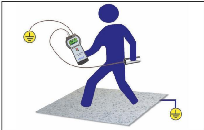
Figure 3. Setup of the Body Voltage Meter
