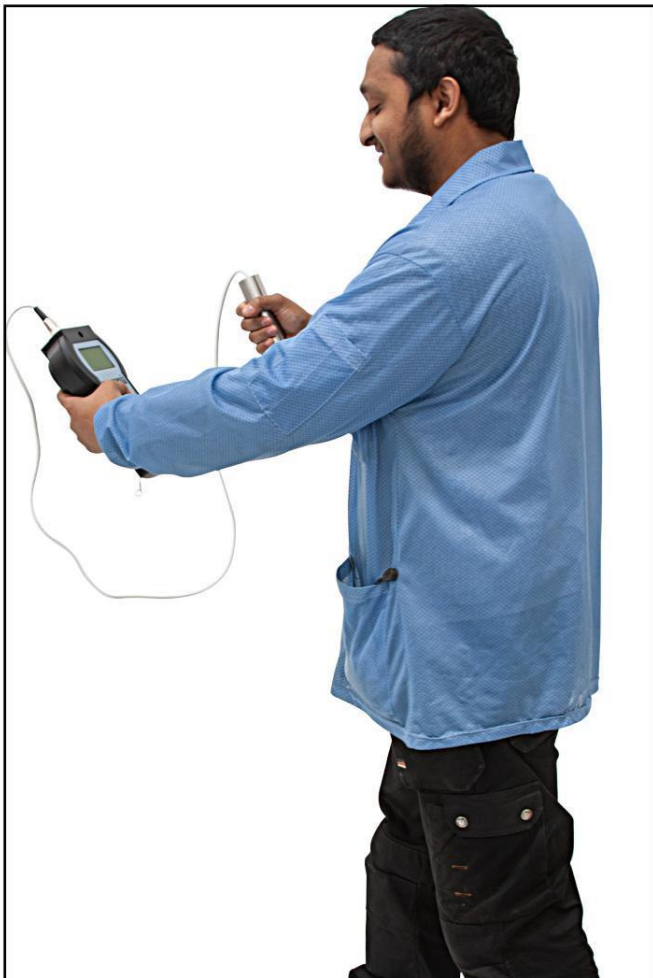
Figure 5. Using the Body Voltage Monitor
