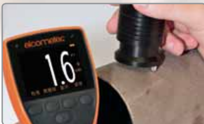
整体式分体式探头测得的粗糙度高达500μm (20mils)
